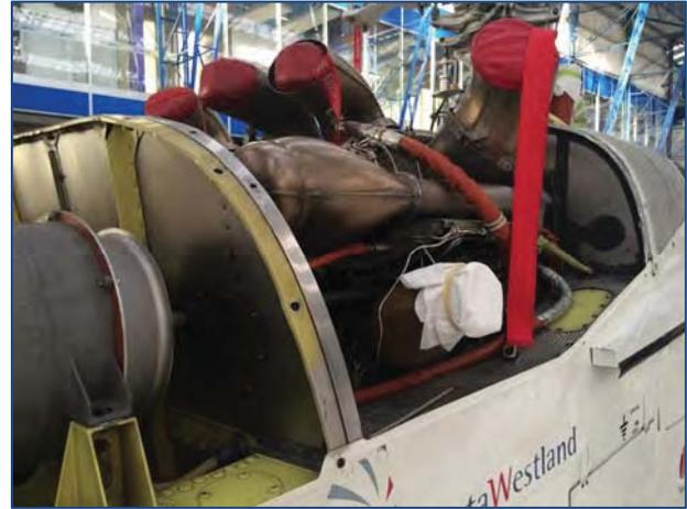
General Visual Inspection TRDS, TGB & T/R Rotating Controls without discrepancies noted. Also borescope inspection was performed inside the Tailboom, torque check to Fuselage-Tailboom attachment bolts with satisfactory results.
