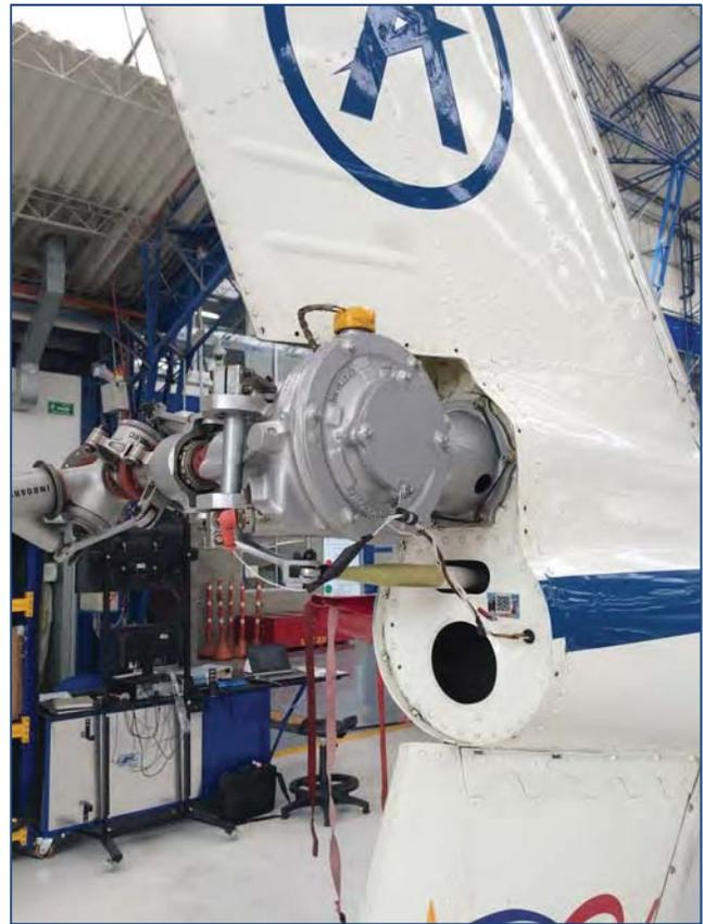
Landing Gear extension/retraction test (4 cycles) performed without discrepancies noted.
