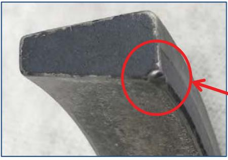
Damage on Lower Conical ring set P/N 109-0101-21-1 S/N A0128, replacement required
