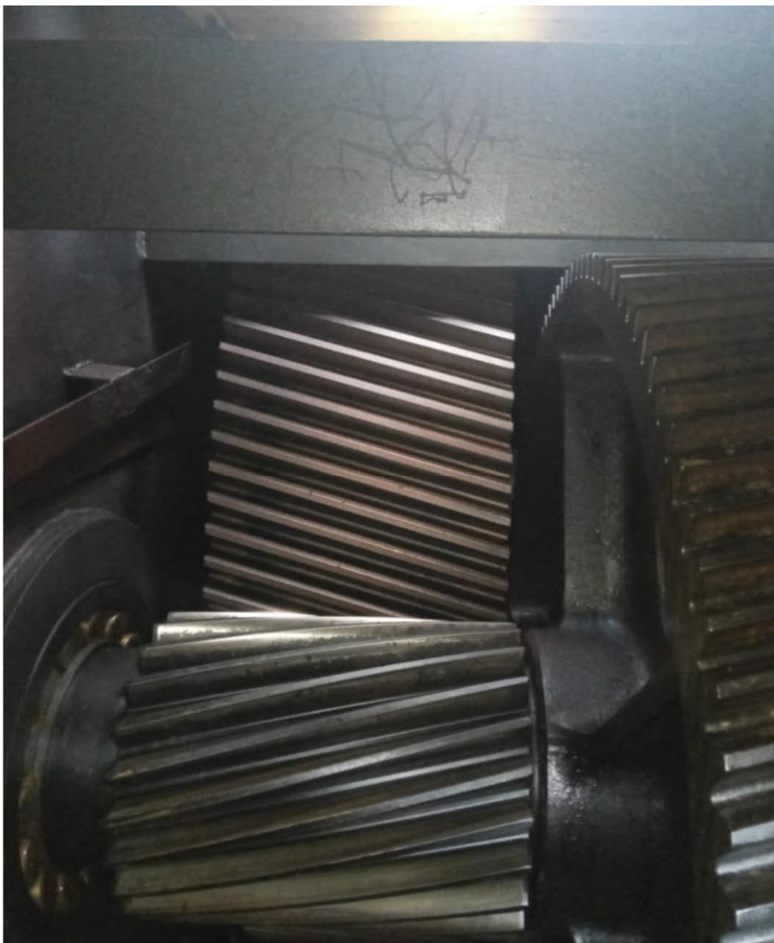
Photo No 5 (Low Speed gear and pinion speed reducer MO # 679-01
